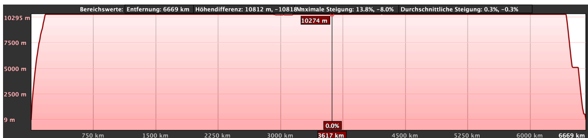
Figure 4: Flight profile. Except for start, landing, and the Lidar leg HALO stayed at FL 320.
