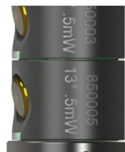
Close-up of LED module engraving showing serial number, pitch angle and optical power. Downward pitch orientation is clearly visible. Note: Quartz tube not shown.
