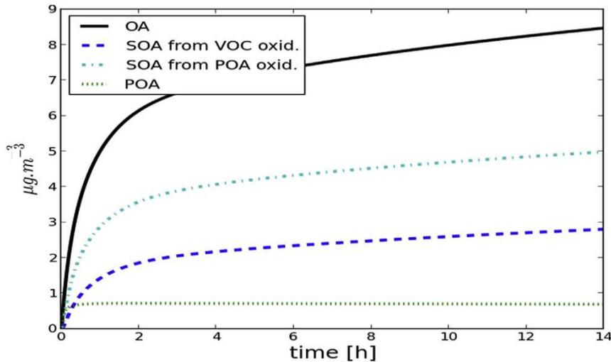
Organic concentrations from ageing of gasoline vehicle emissions (simulation of the experiments of Gordon et al. 2014). Source: Sartelet et al. Atmos. Env., 2018
