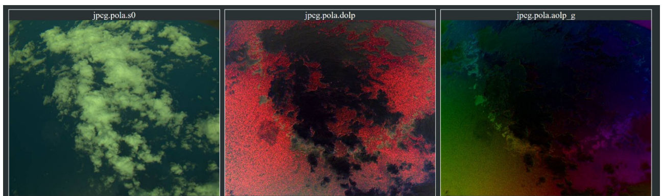
Fig. 11: Observation of a cloud bow (left: radiance unpolarized, middle: degree of linear polarization, right: angle of linear polarization).
